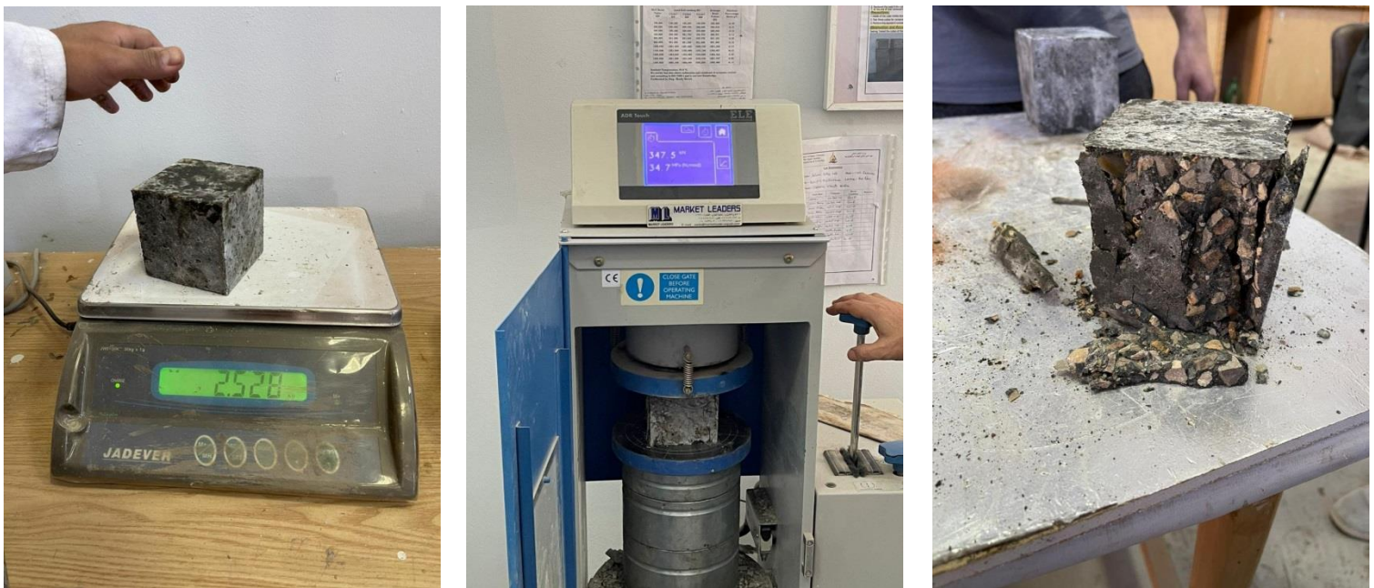
Fig 8.13 weighing and testing cubes on a pressure device
