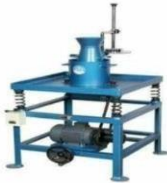
Fig 5 : VEE-BEE CONSISTOMETER TEST
