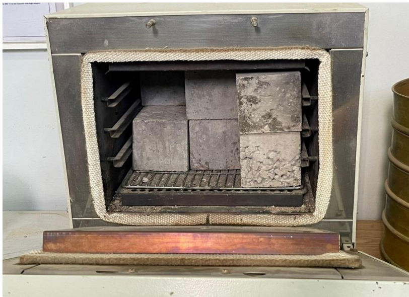
(c) Fig 8.14 heating the cubes and crushing them on the testing machine
