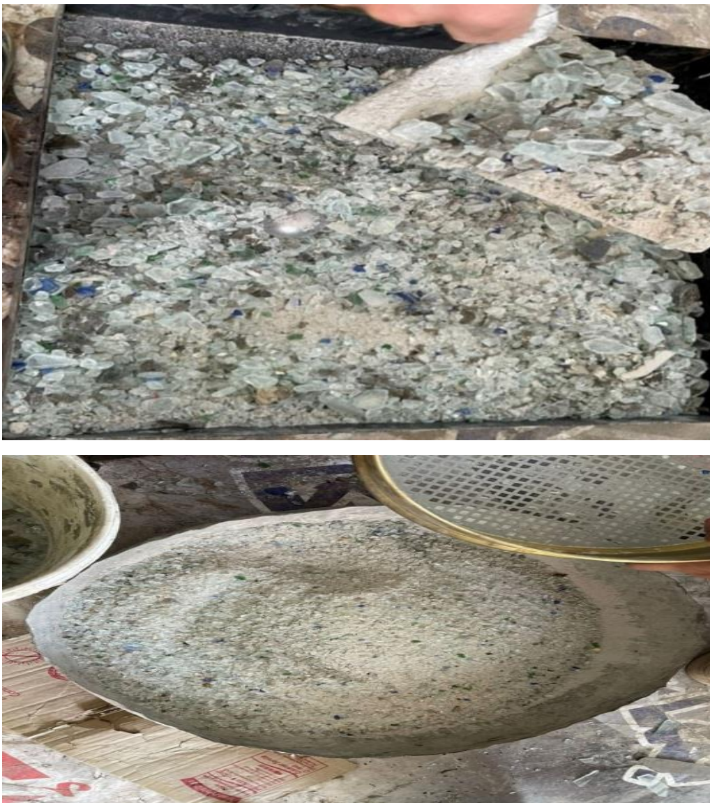
Fig 8.5 place the glass breaking on sieve 4.75
